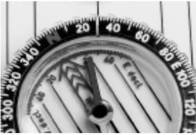
With the declination scale inside the capsule (Field 7, Ranger 3 etc.) turn yourself until red end of the compass needle points to 20 degrees. on the "E. decl." scale – now the direction of travel arrow points in the correct direction.
