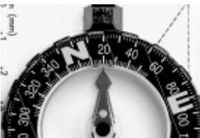
With compasses that have a declination adjuster, (Voyager 9020, 8010 and 8040 etc) you simply hold the graduation ring and turn the compass capsule until the red end of the North arrow points towards 20 degrees. on the Eastern side of the declination scale. When this is done the compass will automatically adjust the bearing. Remember though, to use the North/South lines on the graduation ring as map North reference lines when taking the bearing on the map.
